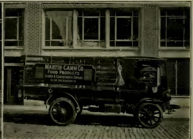
Model 27H, 4-cylinder Autocar. 114 inch wheelbase. 2-3 ton with overall carrying capacity of 15,000 pounds, turning circle 38 feet.
